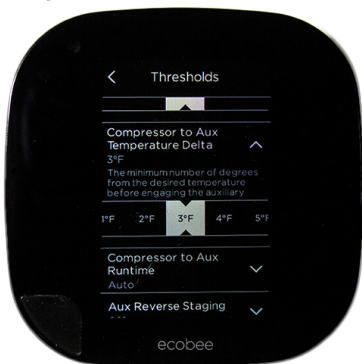
Compressor to Aux Temperature Delta
